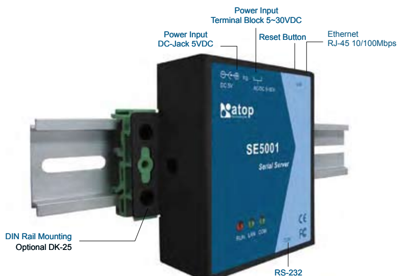
SE5001 DIN-Rail Mounting
